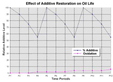
The additives start the next cycle from a very high level and the same scenario takes place. Again a very small amount of oxidation takes place. The oil is reclaimed again and the additives restored. <u>The net</u> <u>effect is that oxidation is controlled at very low levels, water and contaminants never build up to</u> <u>troublesome levels, Oil Life can be extended MANY TIMES!</u>
